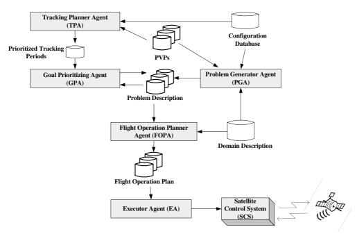
Figure 2. Multi-Agent Ground-operation Automation architecture (MAGA architecture)
